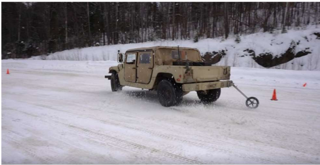
Figure 7: HMMWV testing of lateral acceleration during the slalom test on packed snow and ice.
