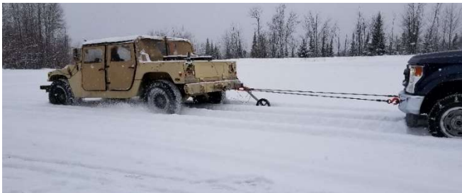
Figure 2: Drawbar Pull testing in 20 cm of fresh snow, Jan 2021.
